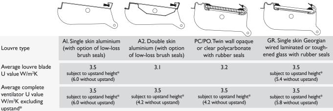
\* In many cases a U value of at least 3.5 W/m<sup>2</sup> is required to meet the Building Regulations. This value can be achieved or surpassed if the ventilator is installed on an upstand which protrudes above the outer membrane of the roof. Colt can advise on this.
