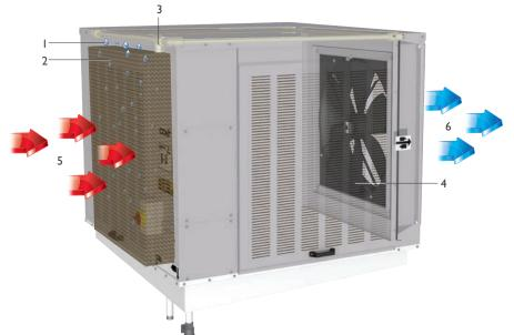
Hot external air (5) is drawn by an axial fan (4) over a desorption medium (2). This medium is kept continuously moist by the water supply system (1), (3). Combined with either natural or mechanical ventilation, this can result in a great reduction in air temperature (6).
